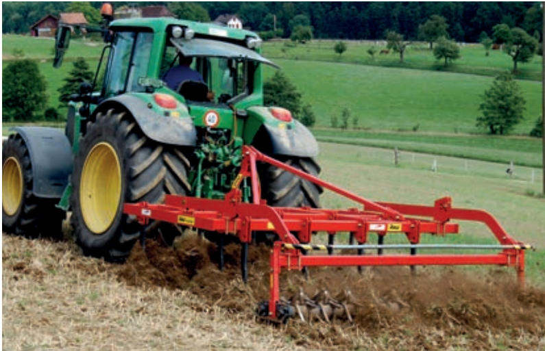
This cultivator with a double-star roller is an alternative to the disc harrow. It loosens the soil in a deep or shallow manner. The machine offers the option of mountable straw feeder and harrow for an optimal incorporation of straw.
