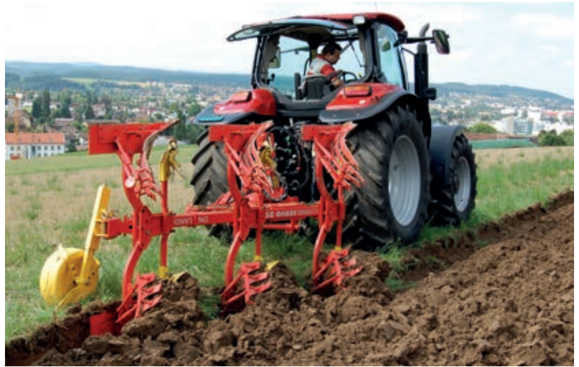
The on-land plough can drive outwith the furrow. The as yet uncultivated soil sustains less damage from driving. Slippage and the creation of a plough sole can be avoided. The usual rules of practice against soil compaction still apply for the on-land plough.
