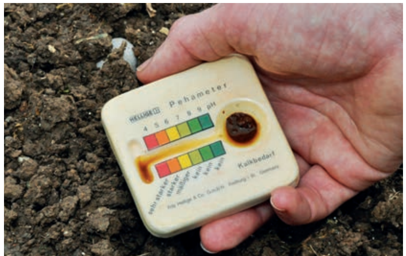
The Hellige pH-Meter combines the soil with an indicator solution, and the level is shown on a colour scale.
