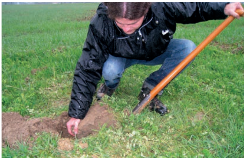
Taking spade tests requires a lot of care. The soil brick should not be damaged during digging. During lift-out, the soil brick needs to be held, to prevent it from breaking apart.
