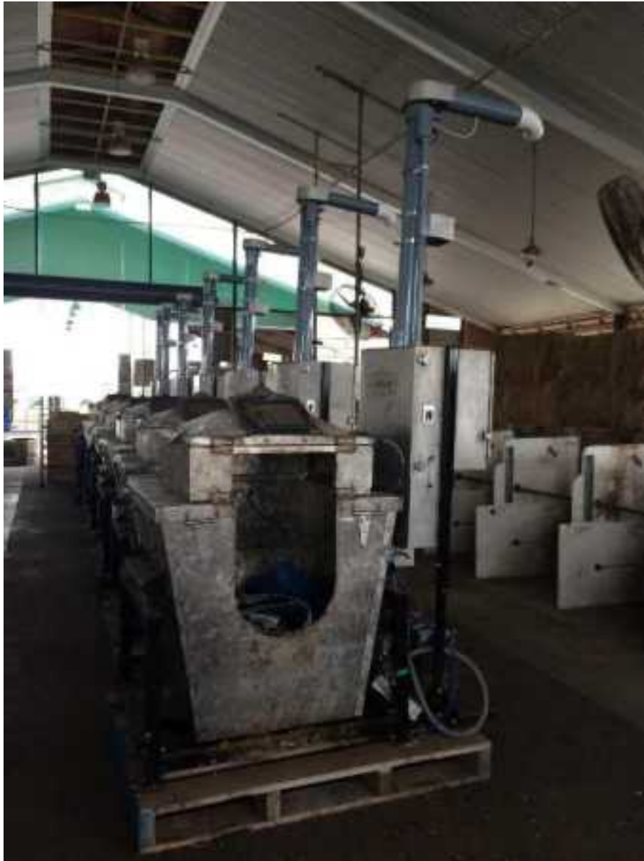
Figure 39: Apparatus to measure methane from cows
