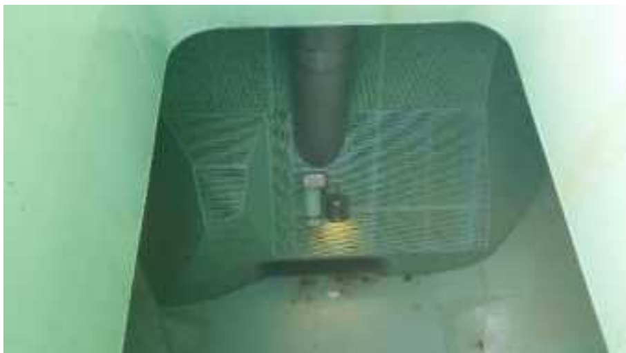
Figure 7: Hull of well boat. Fish are transported to and from sea within the hull of the boat. Medicinal treatments are also administered in these boats.
