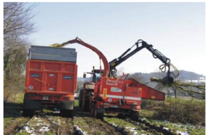
Whole tree chipper in operation. Previously the hedge had been coppiced and the trees and bushes laid in a line beside the hedge. 100m of hedge can be chipped in one hour! St. Amand, Normandy, February 2012.
