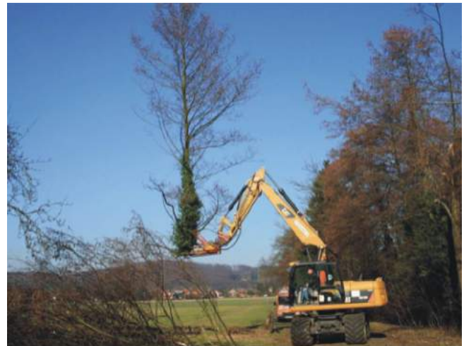
Hedge tree felled and being lifted clear by an excavator with feller-buncher head. Kries Steinfurt, Germany. Photo: Benedikt Brinkt.
