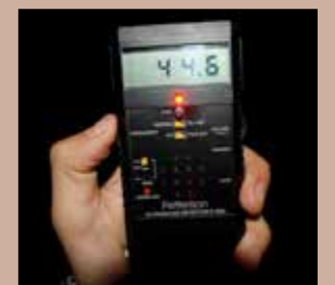
Bat detectors identify bats from their unique high frequency calls © Gilles San Martin CC BY NC 3.0
