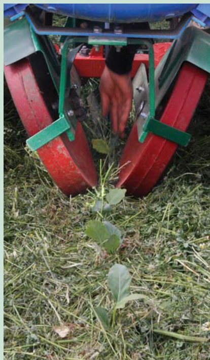
Brassicas being planted with the MulchTec planter
