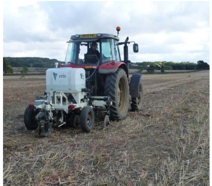
Figure 9. Soil electrical conductivity (EC) scanner
