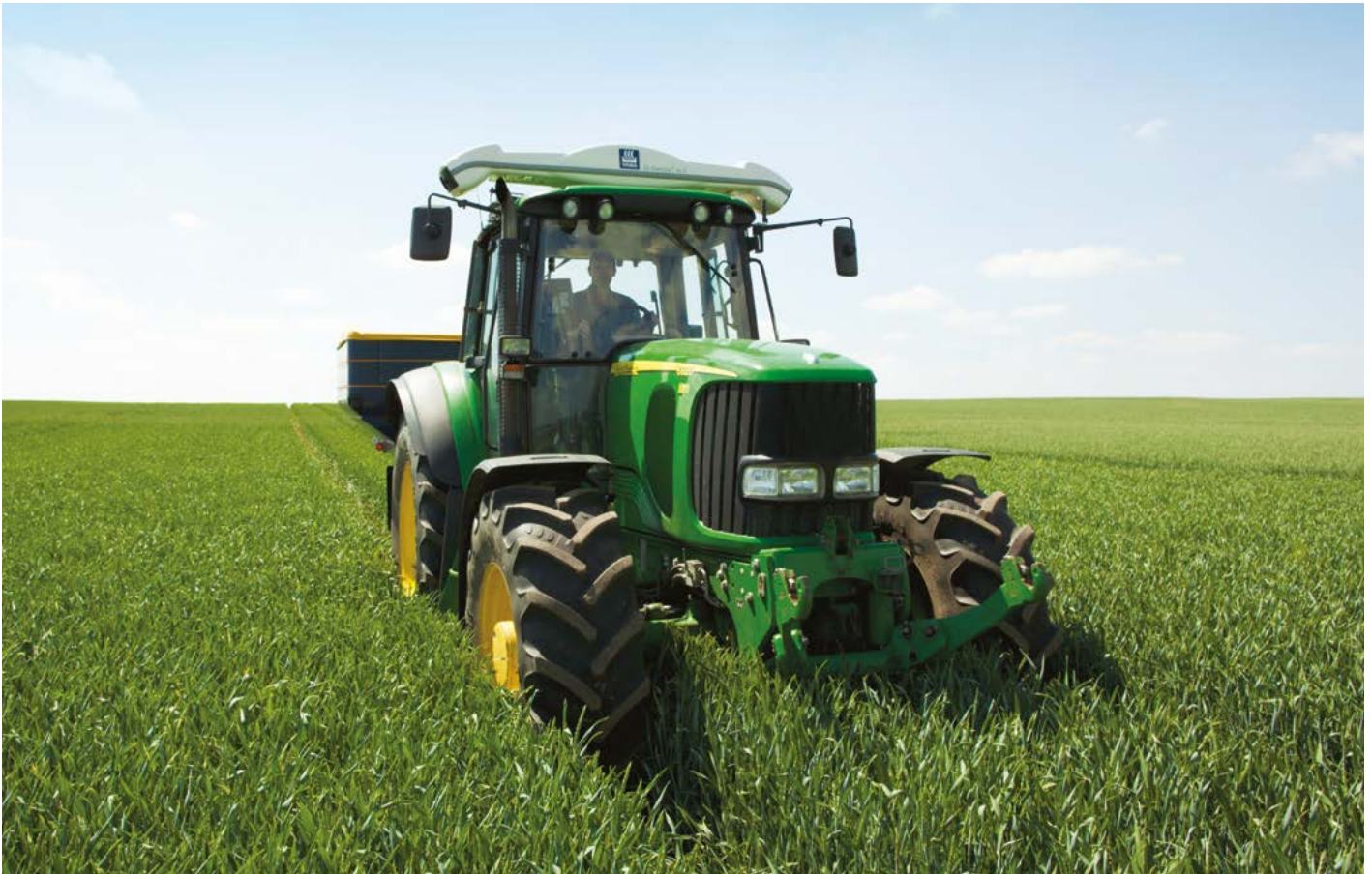
Cab-mounted Yara N-Sensor controlling fertiliser spreading rate in real time
